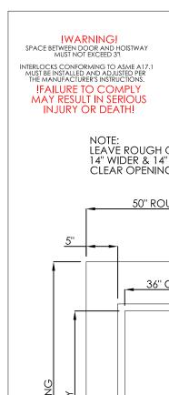
NOTE: LEAVE ROUGH OPENING MIN 14" WIDER & 14" HIGHER THAN CLEAR OPENING, AS SHOWN.
